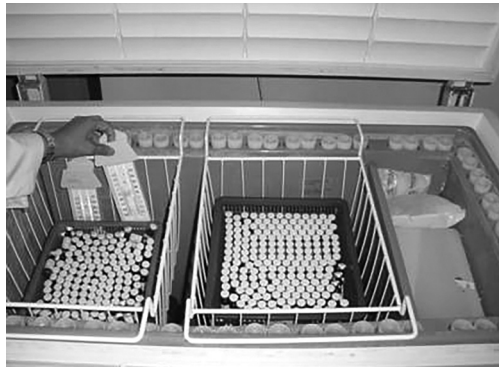
Fig. 2: Vaccine storage in ice-lined refrigerator.
